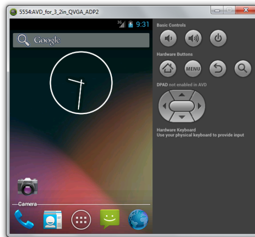
Figure 4: An Android Virtual Device (AVD) running on local port 5554.
